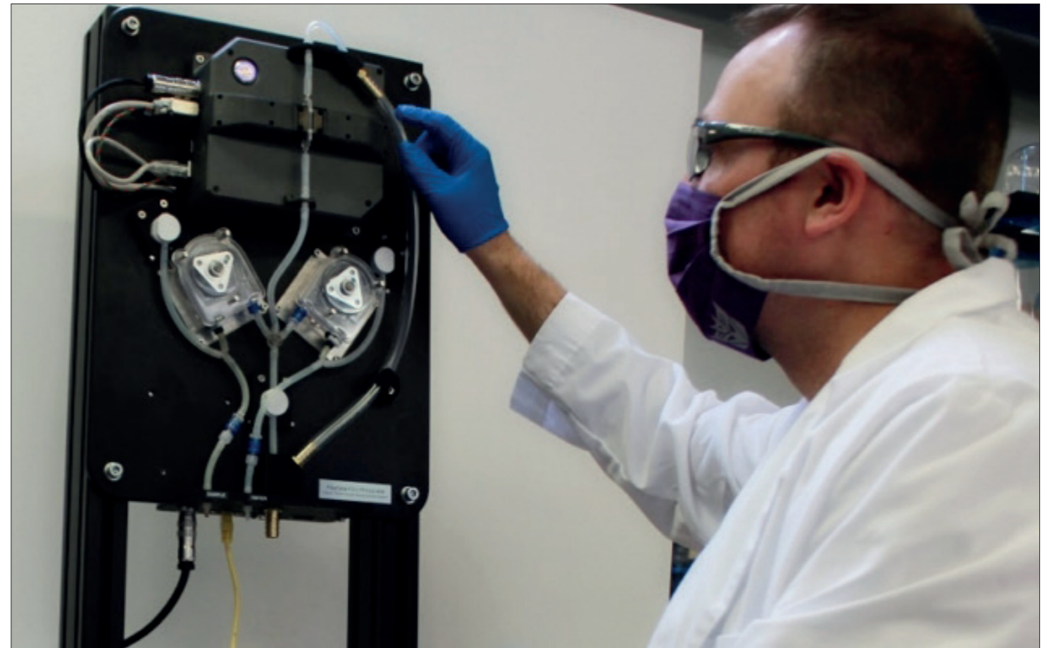
Optical know-how: an LTMS test assembly at Ocean Insight's Rochester, NY, development facility. When deployed into an industry setting, the LTMS can generate high-precision colour and concentration measurements on a 24/7 basis. (Courtesy: Ocean Insight).
